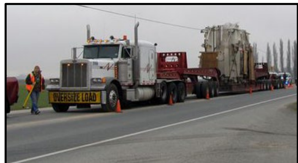
Super-load requiring bridge loading analysis.
